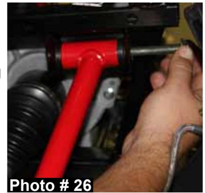
34. Attach the lower shock eyelet to each new Skyjacker upper A-arm using the OEM hardware & a 15mm socket. (See Photo # 27)
