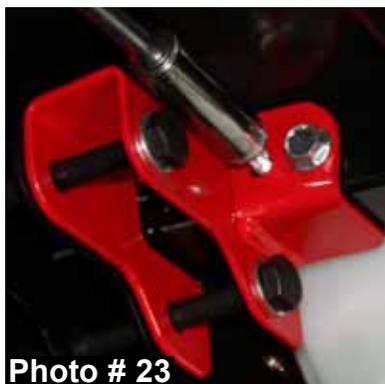
31. Remove the 10mm x 100mm bolt, washers, & nut that are to the inside of the frame on each new Skyjacker upper shock bracket & install two of the new Skyjacker sleeves (Part # CS1281) into the two inside upper shock mounting locations. Reinstall the 10mm x 100mm bolt, washers, & nut through each new Skyjacker upper shock bracket & new Skyjacker sleeves using a 17mm socket. **Note:** Do not tighten at this time. (See Photo # 24)
