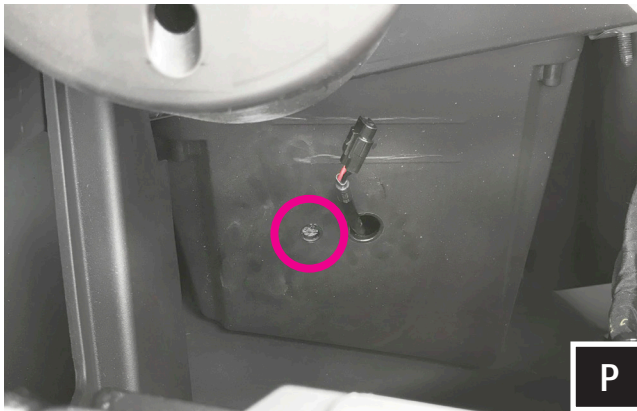
P. From the inside-top of the dash, secure the top mounting M6 screw and large washer to the pod through the smaller hole next to the routed speaker wire.
