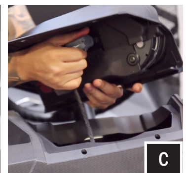
C. With push pins extracted, lift to remove the cup holder and gauge cluster.
