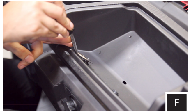
F. Extract push pins that are now exposed from removing the upper glove box.
