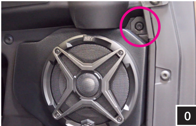
O. Place the speaker pod in location and resecure the factory screws through the pod brackets on the front and underneath the dash.
