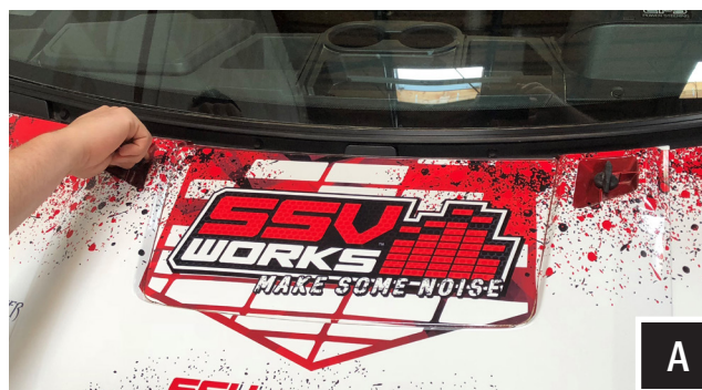
A. Remove hood by turning locking pins and lifting up.
