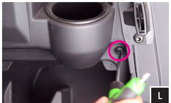
L. Remove factory T40 torx screws located from the front of the dash next to the cup holders.
