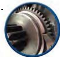
External disc brake prevents damaging heat to synthetic rope
