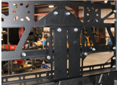
FIG 17 - Assemble Spare Tire Mount using 13mm Wrench and 13mm Socket
