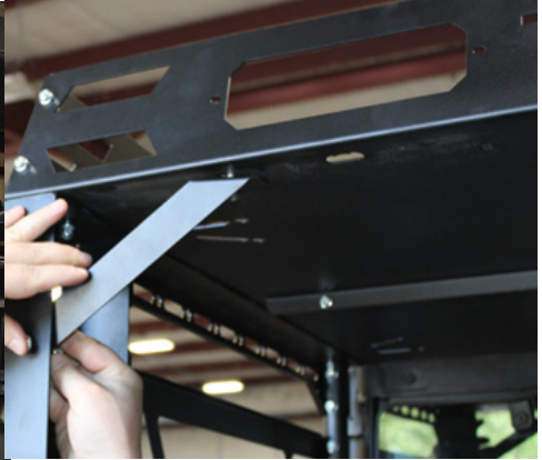
FIG 16 - Use 13mm Socket and 13mm Wrench to install Sway Supports (12 & 13)
