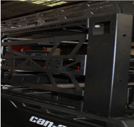
FIG 15 - Secure Upper Front and Rear Racks using 13mm Socket and 13mm Wrench
