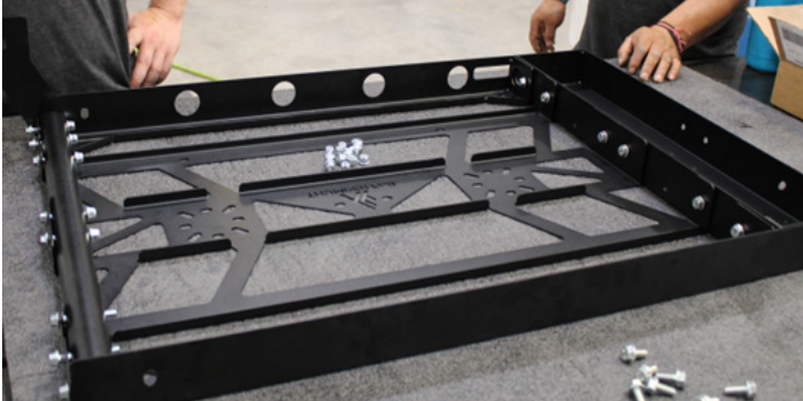
FIG 2 - Hand Tighten Hardware for Each Side
