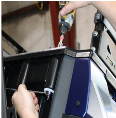
FIG 5 - Using 7/16" Socket & 7/16" Wrench Install Washers to Front Corners of Bed
