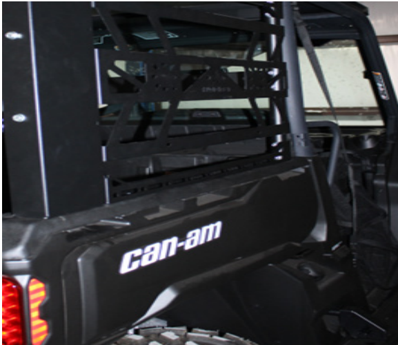
FIG 3 - Put Loosely Assembled side Rails on Bed
