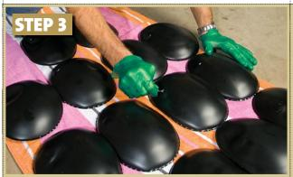
**PREP THE TIREBALLS.** Lay the TireBalls out on a clean, flat surface and place a dab of silicone needle grease on the inflation valve of each TireBall. This will expedite the process of inserting the inflation needle into each one. Also at this time, we partially inflate the balls with a three- to four-second burst of air from the TireBalls' standard inflation regulator. This makes it easier to place them loosely in the tire carcass.
