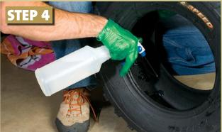
**LUBE THE TIRE CARCASS AND TIREBALLS.** Spray the inside of the tire liberally with some silicone Ball Lube. Next you'll want to rub the lube into the carcass of the tire, making sure to cover the whole inside of the tire. After that, cover each of the TireBalls with the silicon Ball Lube, making sure not to leave any part of it dry. This is why we mention you'll want to wear old clothes ... this is when the steps start to really get messy!
