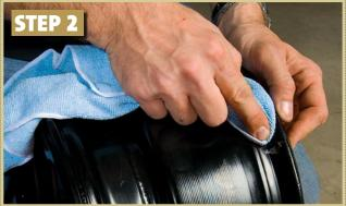
**PREP YOUR WHEEL.** Clean the inside and outside of the wheel and check for any burrs in the aluminum by rubbing a cloth over it. If the cloth snags, you must de-burr it with a piece of fine-grit sandpaper. Follow up by thoroughly recleaning the wheel. If you miss this step, the TireBalls could end up toasted before you ever get a chance to abuse them. You definitely don't want them to snag or tear themselves on any sharp burrs in the wheel!
