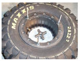
10) After removing the Bead Hold Down Clamps, apply additional bead lube onto the exposed tire bead and rim. Laying the wheel flat on the ground, attach an inflation hose to the valve stem (core removed) and inflate to seat the tire beads onto the rim.
