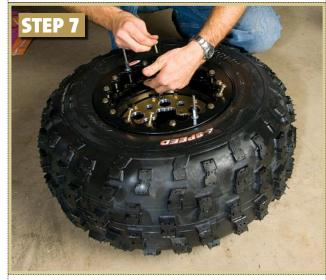
**SECURE THE BEAD LOCK.** Line the bead-lock ring up with the wheel and draw it tight with the bead-lock stud kit. We chose to arrange the stud kit in an equilateral-triangle pattern to more easily and more evenly mate the bead-lock ring with the wheel. Once you have the ring and wheel drawn close enough for the bead-lock studs to reach the wheel, run those in and tighten them to the recommended torque specs.
