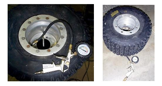
For your own personal safety, never use an air chuck applied to the valve stem, use a remote inflator as shown.
