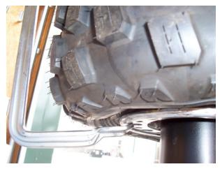
10a) For Bead-Lock Wheels - Use three long studs screwed into equally spaced holes around the rim. Install the bead lock ring and pull the ring down gradually until the bolts supplied with the rim can be started by hand. Tighten the bolts and replace the long studs with the remaining bolts supplied with the rim.
