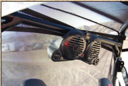
INSTALLED ROLL BAR MOUNT REAR OF POLARIS RZR
