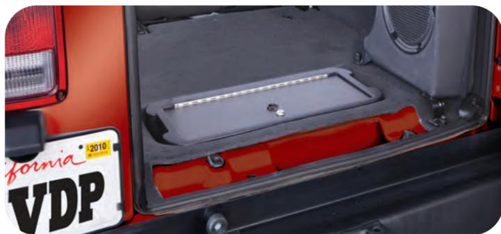
Keeps valuables safe and secure when top is off and doors unlocked. Discreetly hidden below rear cargo floor carpet. Quick and easy installation securely bolting to existing Jeep body vault. Crafted design with 16 gauge steel lid and stainless steel piano hinge makes it impossible to pry open.
