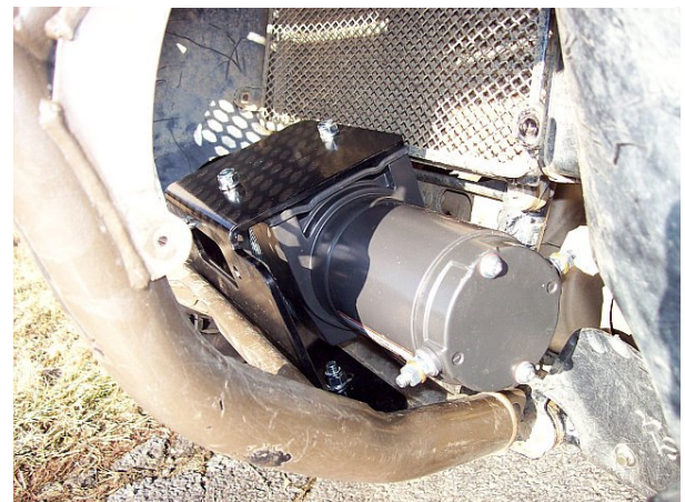
"Figure 2" Mount Shown in Position with winch
