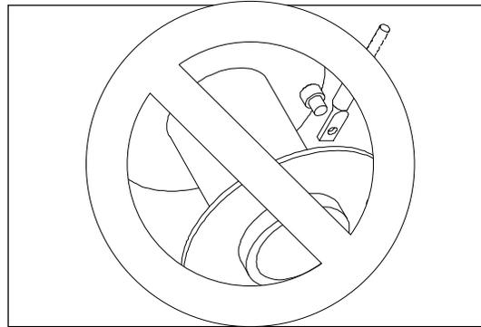
If wire rope has a terminal on the end, it must be cut off before installing.
