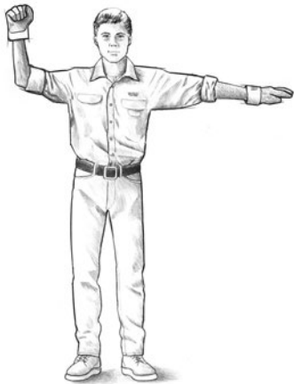
5) Stop the winch Clinch fist, palm to driver, held high enough for driver to see and other arm straight out at shoulder height is the sign to stop the winch.
