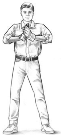
6) Braking Cross your palms together to tell the driver to apply the foot brake.
