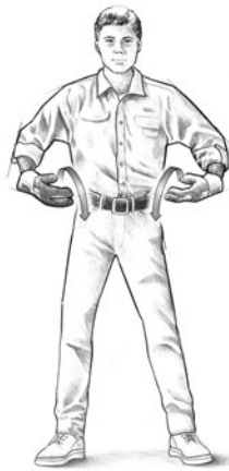
7) Drive assist Tells driver to give the tires more drive force to assist the winching process.
