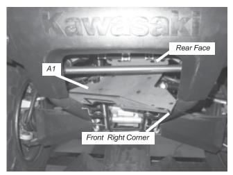
Figure 3 Rear Support Mount Bracket
