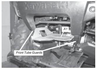
Figure 2 Install Winch Mounting Plate
