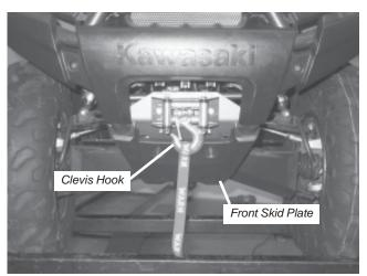
Figure 7 Complete Winch Installation
