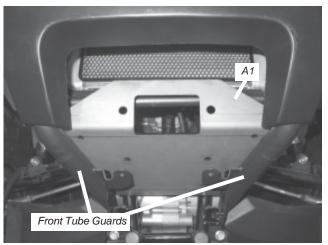
Figure 4 Place Winch Mounting Plate into Location
