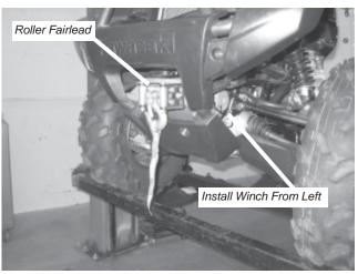
Figure 6 Install Winch and Roller Fairlead
