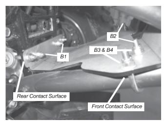
Figure 5 Fasten Winch Mounting Plate
