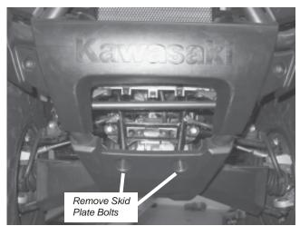
Figure 1 Loosen Front Skid Plate
