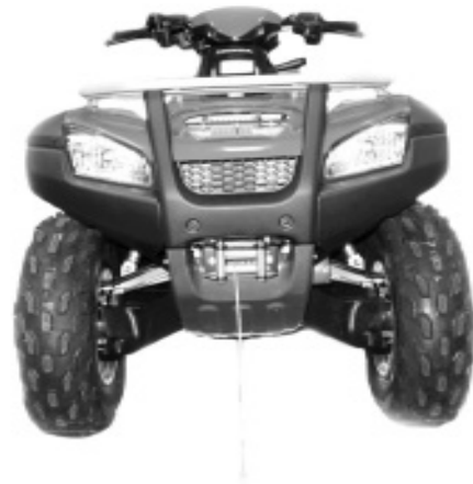
Figure 8 Completed Winch Installation on Rincon
