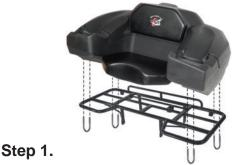
Place the cargo box or the cargo box seat on the rack to identify the best location to install the «U» bolts.
