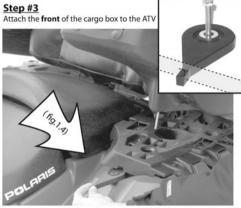
Slide an anchor under the rack on each side and place the cargo seat on the rack. (fig.1.4) Screw on the bolts but do not tighten completely for now.
