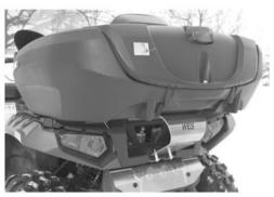
Complete the installation by tightening the bolt and the 2 front bolts.
