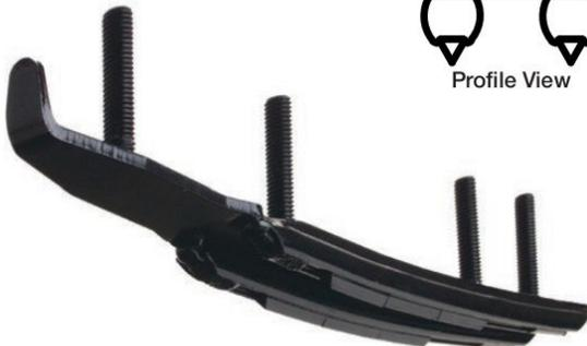
The Dooly™ runner will help decrease darting of your sled as it makes its own groove in the trail. The tucked front end will ensure stability. The two 7/16" Flat-Top® runners mounted on a plate are available in 4", 6", or 8" of 60° turning carbide to accommodate several styles of trail riders. Each Dooly™ runner is packaged individually.
