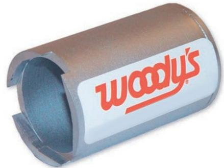
Align your Triangle Digger® support plates by using this specialized indexing tool. To be used with a 3/8" ratchet for 5/16" or 7mm support plates. Part Number: SPI-TOOL-T
