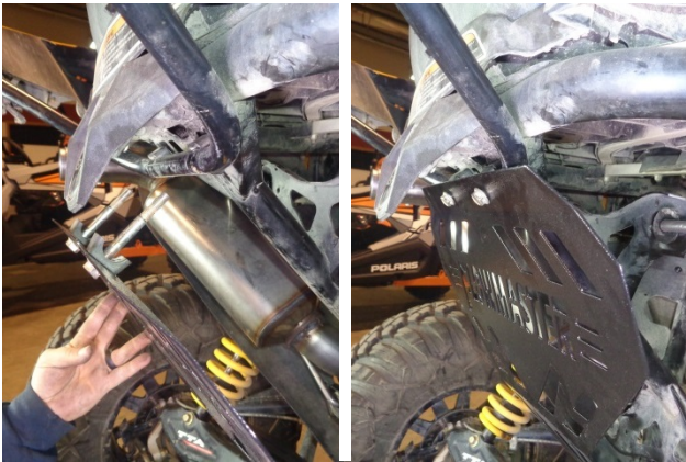
12. Insert the 2 bolts through their holes in the tail-light support tube, then hand-start (but do not yet tighten) the nuts.
