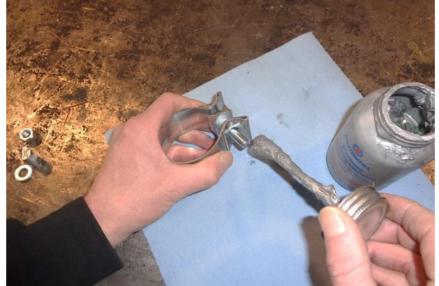
14. Apply anti-seize compound to the bolt threads on the two larger (2-1/4") clamps (2).
