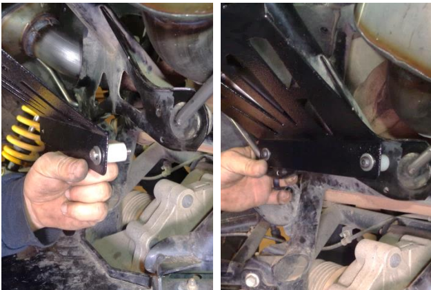
13. Fasten the bottom of the heat shield to the frame at 2 places, using screws (10) and flat washers (7) (on the heat shield side); nylon spacers (6) (between the heat shield and the frame); and flat washers (7), lock washers (8) and nuts (9) (on the frame side). Once both nuts have been started by hand, tighten all heat shield fasteners (4 places).
