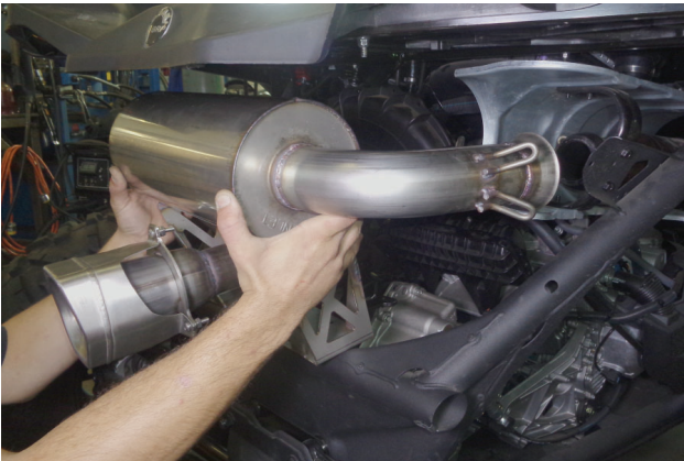
13. Place muffler into place on vehicle.
