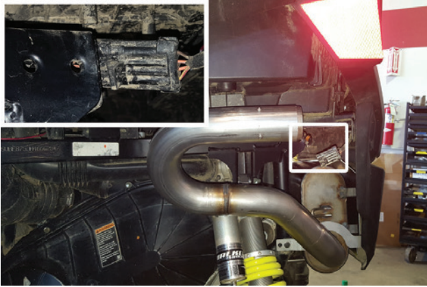
12. Re-connect rear taillight harness as shown.
