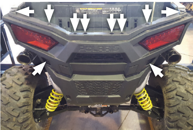
14. Install remaining screws (x10) (removed step 2) to complete fascia install.
