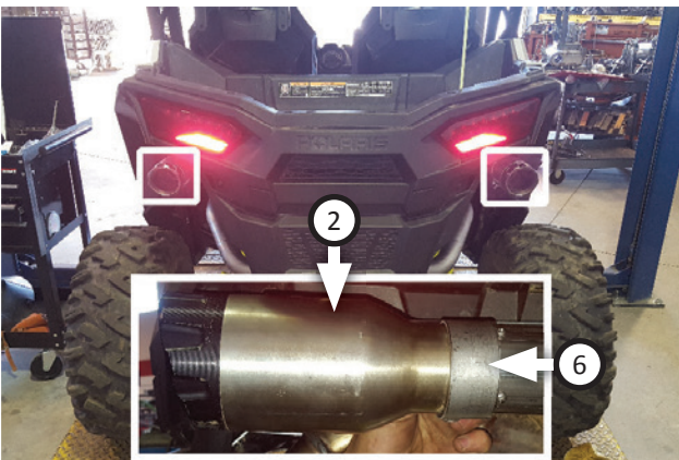
13. Place (x2 ea.) clamps (6) onto exhaust tips (2) then connect them to tailpipes. Tighten clamps to secure connection.
