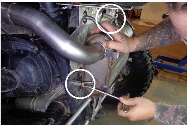
21. Use a spring puller to connect the 2 muffler mount springs to the new muffler.
