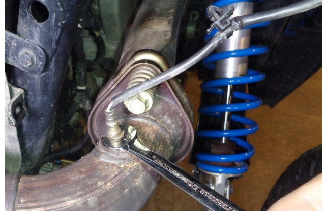
10. Remove the O2 sensor from the exhaust pipe.
