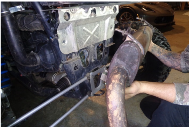
14. Remove the muffler from the vehicle.
