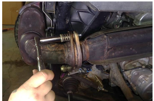
12. Remove the flange bolts.
