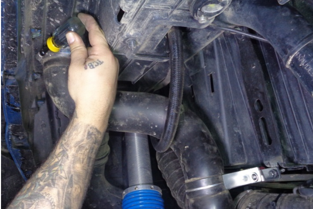
19. Tighten the clamp at the top of the clutch cooling air duct.
