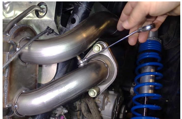
23. Apply anti-seize compound to the O2 sensor threads. (Do not get compound on the tip of the sensor.) Then install the sensor in the exhaust pipe.
