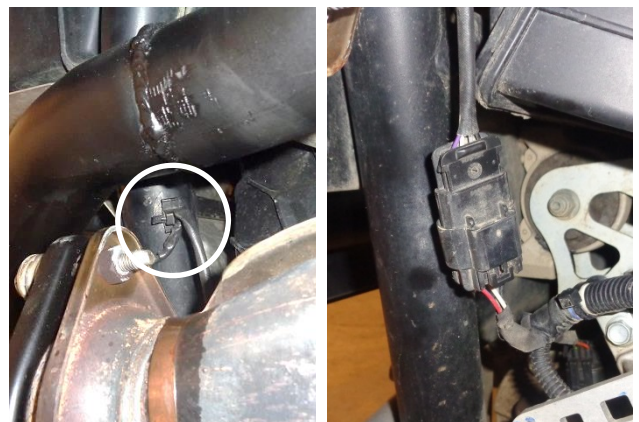
24. Fasten the O2 sensor lead clamp to the vehicle frame. Then connect the sensor lead to the electrical harness, and verify the connection is secure.
