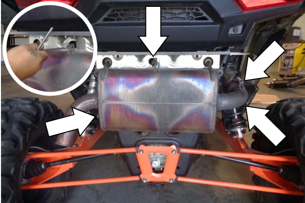
7. Use a spring puller to release the four muffler mount springs.
