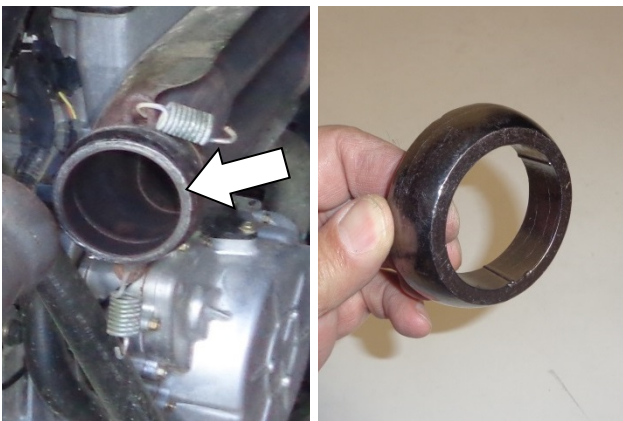
9. Inspect the lead gasket on the end of the exhaust pipe for serviceability. Replace if required.
