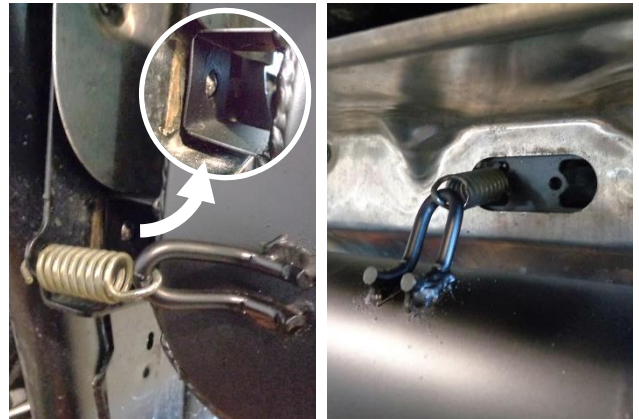
11. At the lower left corner of the muffer, center the alignment hole over the bump on the forward heat shield. Then use a spring puller to connect the 2 muffer mount springs to the new muffer.
