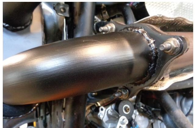
12. Apply anti-seize compound to the 3 flange studs, then install the nuts and tighten them down evenly.
