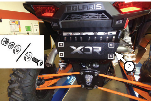
14. Install heatshield (2) over muffler using screws (4), flat washers (5), split lock washers (6) and hex nuts (3). Tighten fastener assemblies completely.
