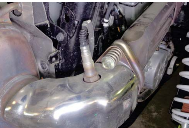
9. Remove the O2 sensor from the exhaust pipe. NOTE: Use penetrating oil to avoid thread damage.
