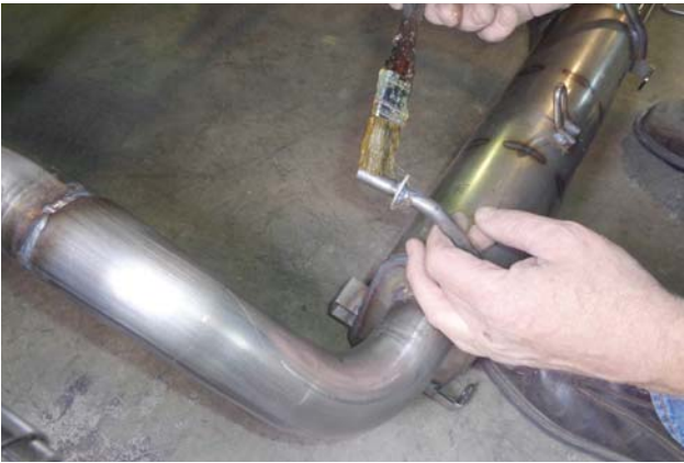
20. Lubricate the 2 hanger pins on the muffer (1) with grease or oil.
