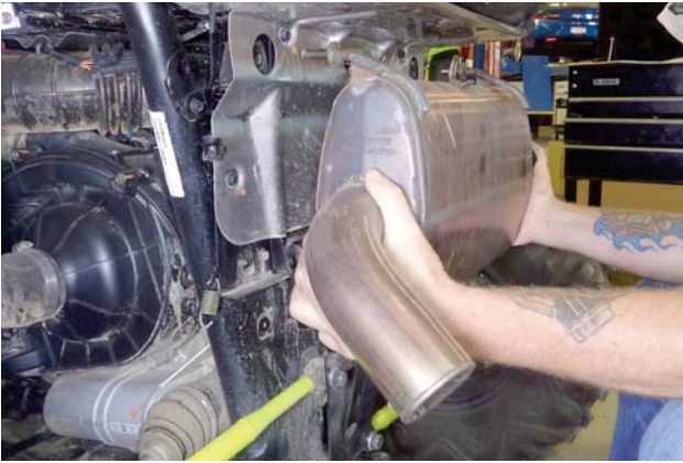
13. Remove the muffler from the vehicle.
