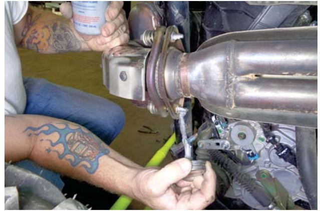
10. Apply anti-seize compound to the exposed threads of the 2 flange bolts to prevent seizing.
