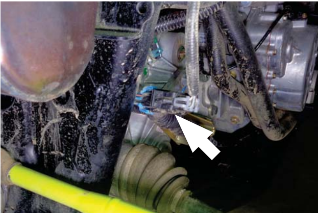
8. Disconnect the oxygen (O2) sensor lead from the electrical harness.
