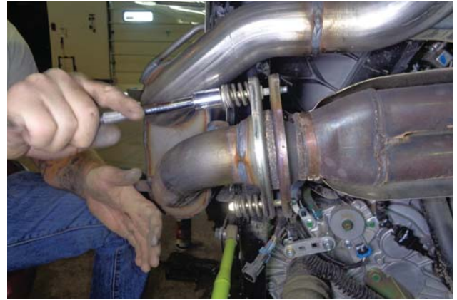
23. Apply anti-seize compound to the two flange bolts, install them, and tighten them down evenly.
