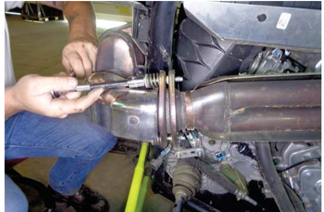
11. Remove the 2 flange bolts.
