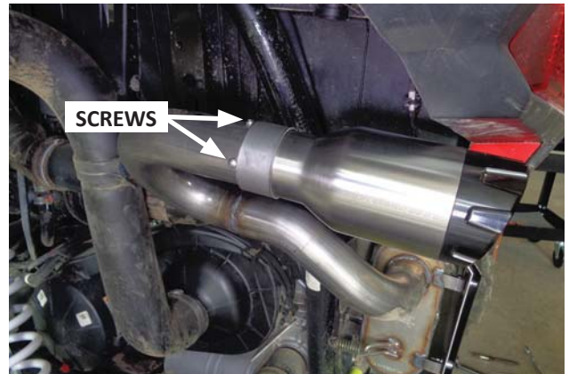
34. Push each tip onto its pipe until its clamp touches the spark arrestor screws. Also be sure to keep the rear edge of the clamp just over the end of the Z-notch (per Step 32). When each tip is in place, tighten its clamp.
