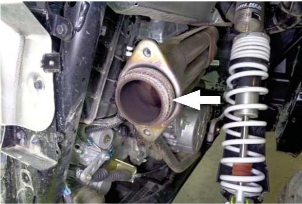
14. Inspect the lead gasket on the end of the exhaust pipe for damage (cracks, etc.). Replace if required.
