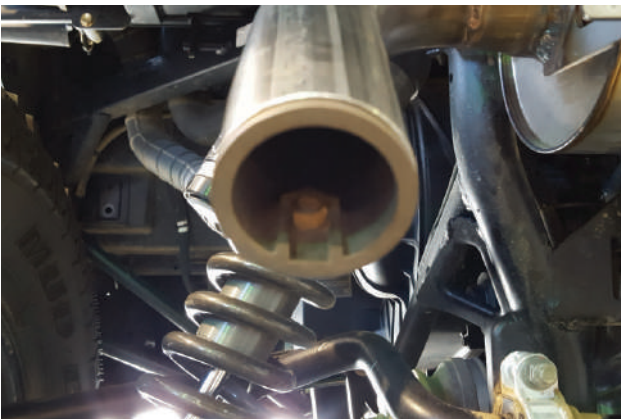
8. Install nut, bolt and spark arrestor (removed step 4) onto muffler outlet.
