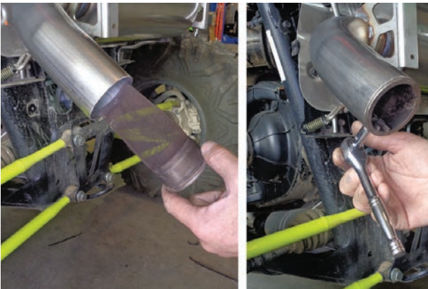
14. Install nut, bolt and spark arrester (removed step 8) into end of muffler.
