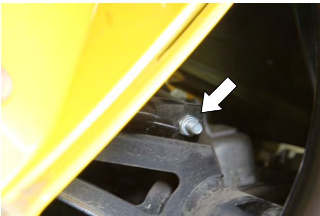
8. Through the gap, locate and remove the stop bolt and nut at the front of the passenger grab bar's right tube. Then remove the 2 grab bar adjustment pins, and remove the grab bar from the vehicle.
