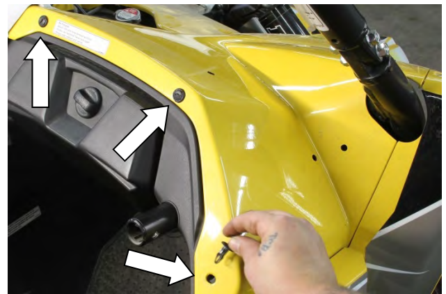
10. Reinstall the 3 plastic push rivets that secure the passenger dash around the glove box.
