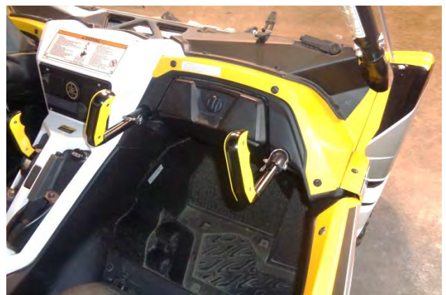
16. Your B&M grab handles can be oriented near-vertical, or near-horizontal. Here, they are oriented slanted slightly inboard from vertical.
