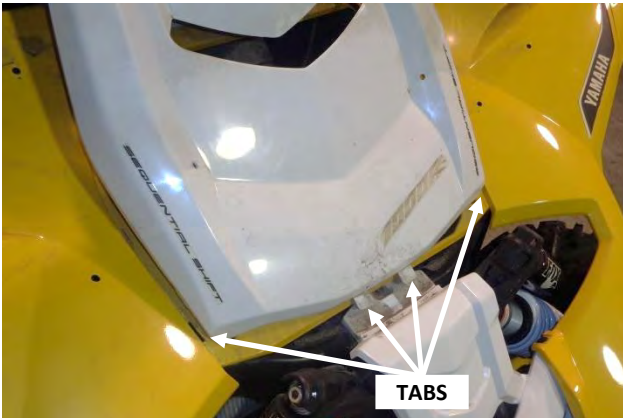
13. Insert the four tabs at the front of the service cover into their respective slots and lay the cover in place.
