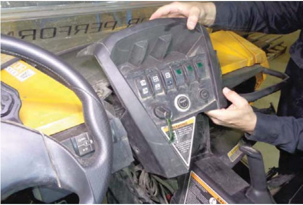
73. Open the glove box and carefully return the control panel to its position on the dash board.
