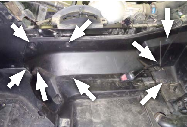
25. Remove the 8 plastic push rivets from the driver side cover panel.
