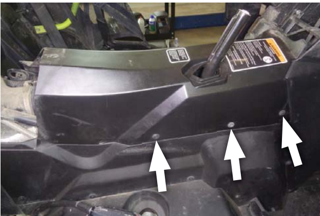
69. Reinstall the 3 push rivets in the right side of the front console.
