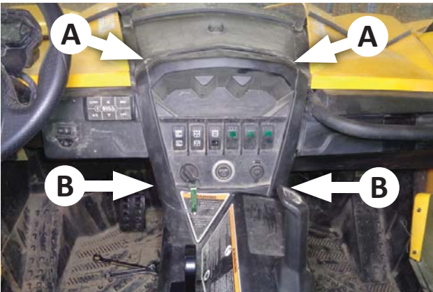
74. Reinstall the 2 screws (A) and the 2 push rivets (B), then close the glove box.
