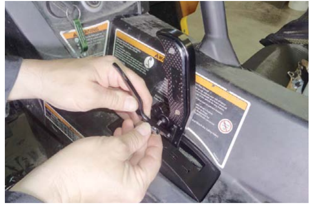
76. Reinstall the trigger lever, spring washer, and shoulder bolt.
