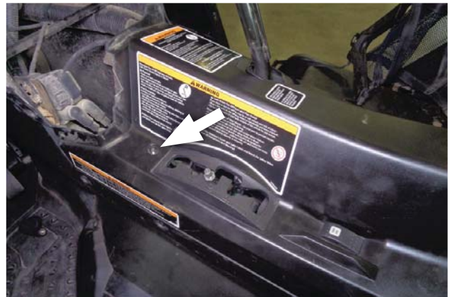
18. Remove the screw from the left side of the front console.
