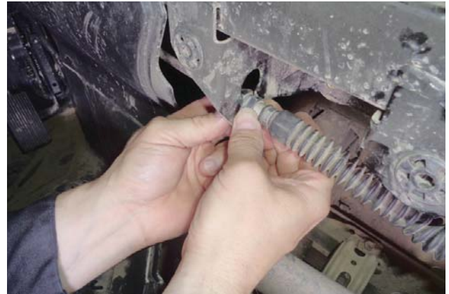
47. Turn both cable adjustment jam nuts back by hand until they are equally snug against the bracket.
