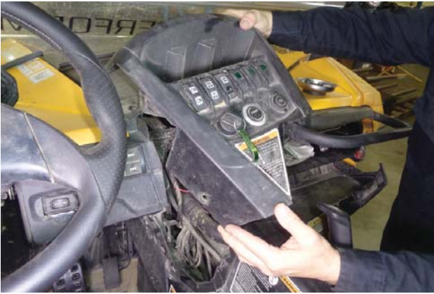
7. Remove the control panel and carefully place it on top of the dash board.
