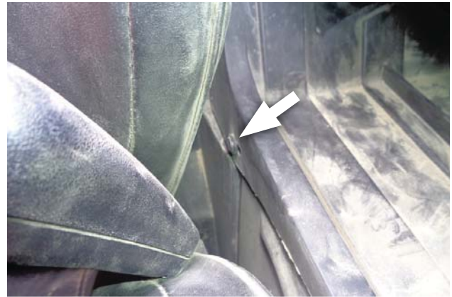
11. Remove the 5th rear console push rivet, next to the right rear seatbelt buckle.
