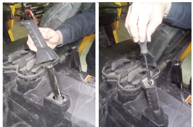
72. Reinstall the passenger grab handle(s).
