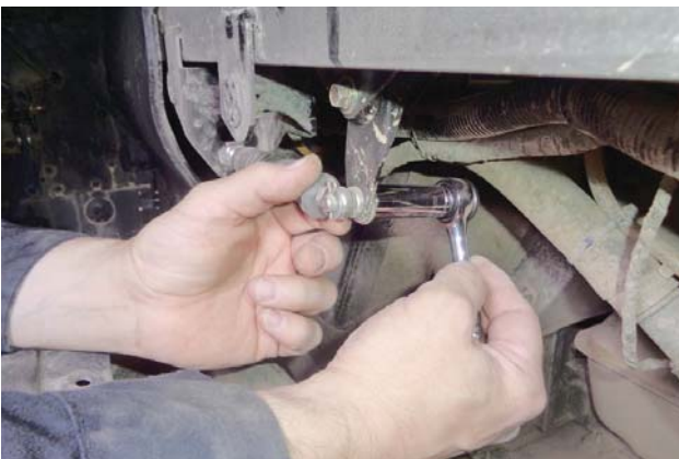
27. Disconnect the shift cable from the shift lever by removing the nut and washer. NOTE: The nut will be re-used; the washer will not be.
