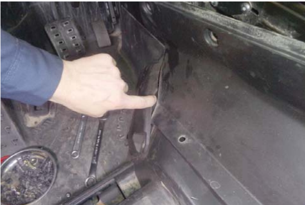
56. Verify that the front bottom corner of the cover panel is tucked beneath the rubber kick guard.
