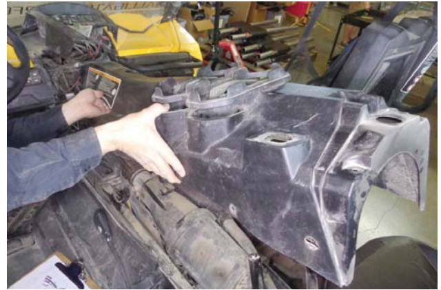
23. Carefully remove the front console cover from the vehicle.
