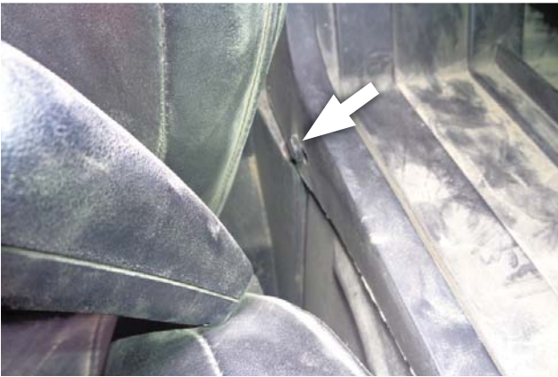
68. Reinstall the 5th rear console push rivet, next to the right rear seatbelt buckle. THEN GO TO STEP 72.
