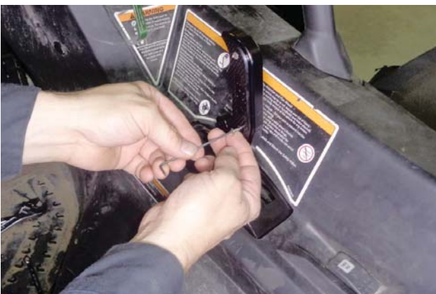
75. Reinstall the 2 grip plates.
