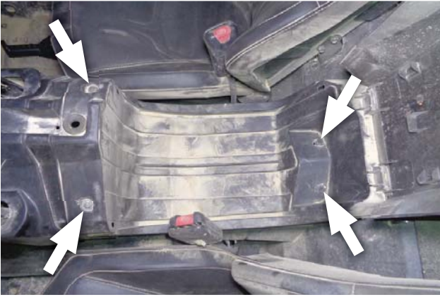
67. Reinstall 4 (of the 5 total) push rivets as shown.
