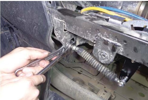
45. Loosen the cable adjustment jam nuts, then back them away from the bracket just enough to allow the cable end screw to reach the hole in the shift lever naturally, without forcing it.
