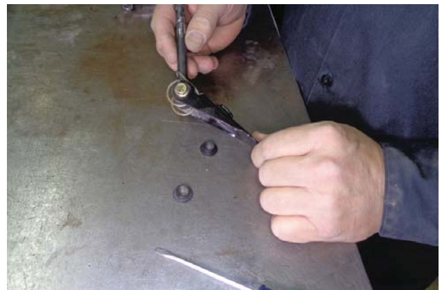
30. Remove the metal sleeve and the 2 plastic bushings from the shift lever. NOTE: The 2 bushings will be re-used; the metal sleeve will not be.
