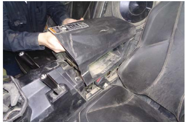
66. Return the rear console to its location in the vehicle, then lift the lid.
