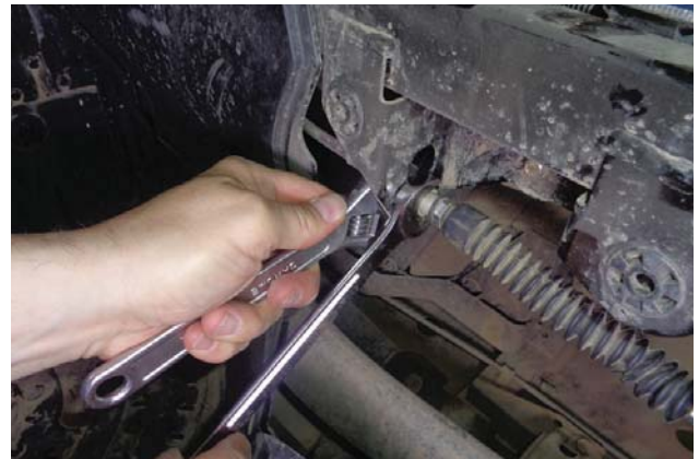
48. Tighten both jam nuts equally against the bracket.
