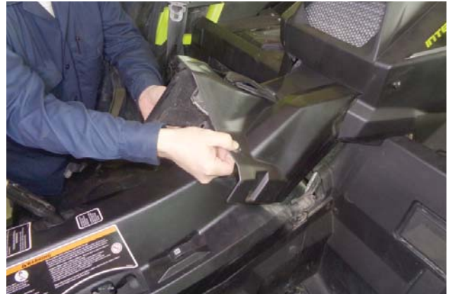
17. Remove the rear console from the vehicle.
