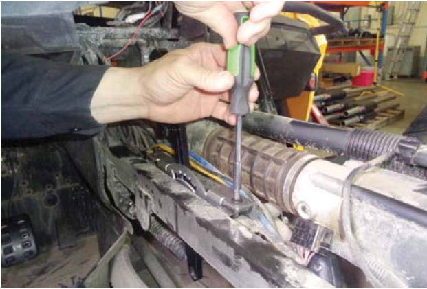
43. Temporarily tighten both shift gate screws.
