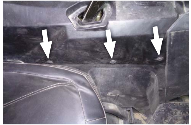
64. Reinstall the 3 push rivets in the front right side of the front console.
