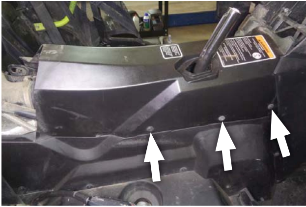
19. Remove the 3 push rivets from the front right side of the front console.
