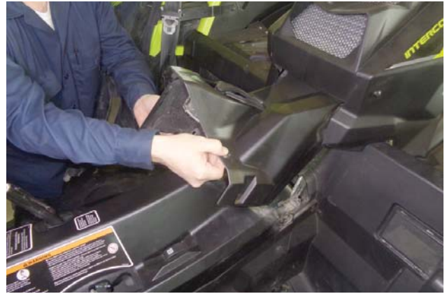
70. Return the rear console to its location in the vehicle.
