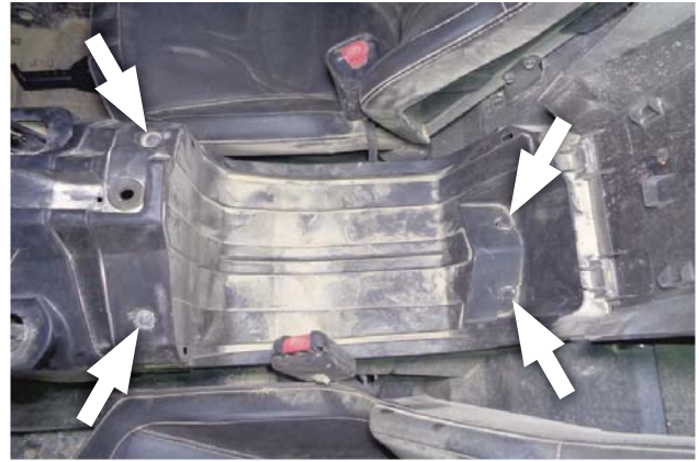
10. Remove the 4 (of 5 total) rear console push rivets shown.
