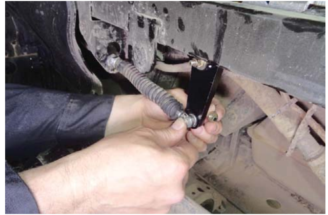
46. Insert the cable end screw in the hole in the shift lever. Make sure that the screw's square profile seats properly in the hole. Then install and tighten the nut from Step 27.
