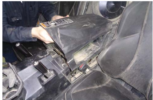
12. Remove the rear console from the vehicle.
