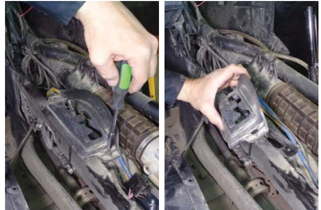
28. Remove the screw and shift gate.
