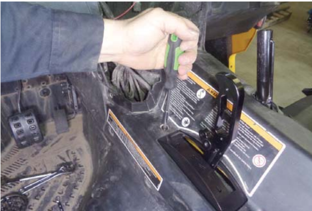
62. Install and tighten the front shift gate screw.
