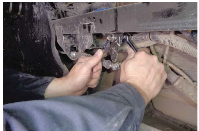
29. Remove the shift lever mount screw, nut, and 2 washers, then remove the lever from the vehicle. NOTE: The the nut and 1 washer will be re-used; the screw will not be.
