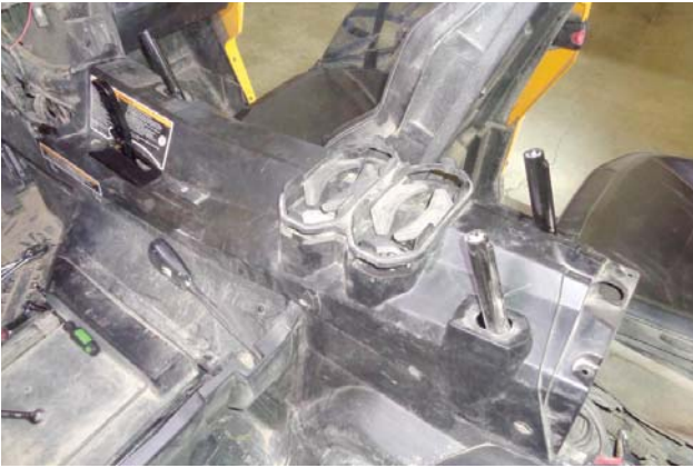
61. Lower the console into place.
