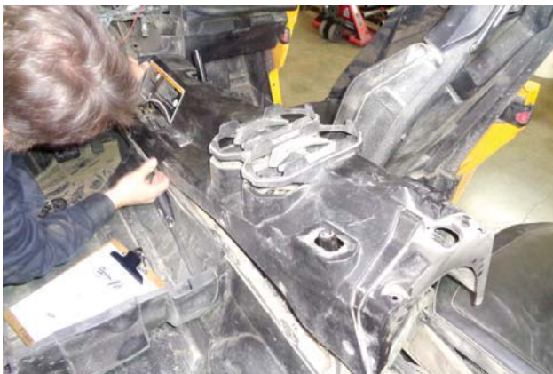
21. Lift the front console just enough to see and reach under it in the next step.
