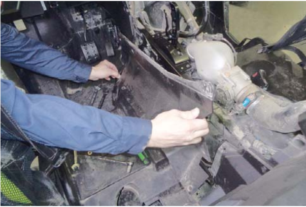
55. Return the driver side cover panel to its location in the vehicle.
