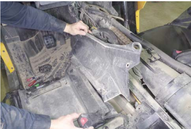
26. Remove the driver side cover panel from the vehicle.
