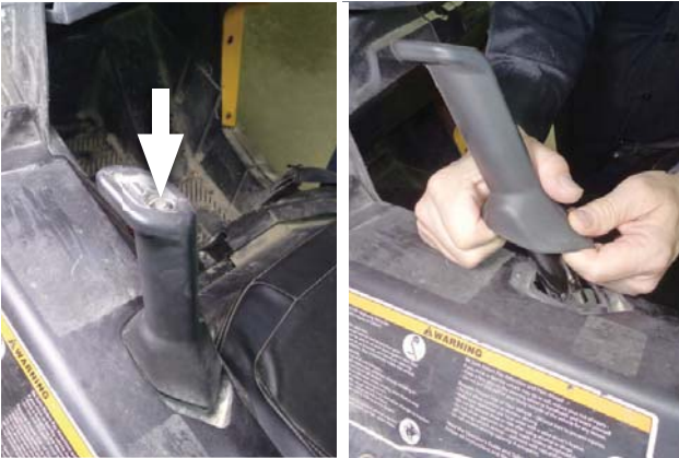
8. Remove the screw(s) from the passenger grab handle(s). Remove the handle(s) by pulling straight up while twisting it back and forth.
