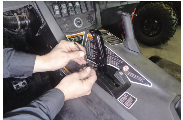
47. Install shoulder bolt, curved spring washer and black lever (removed step 36) onto shifter stick.
