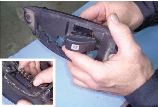
18. Remove override switch (step 12) from factory dust cover (step 11).
