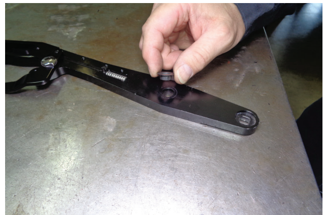
22. Insert plastic bushings (x2) (removed step 16) into both sides of gated shifter stick as shown.
