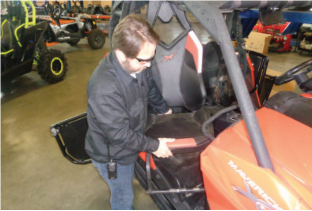
48. Install passenger seat back into vehicle.
