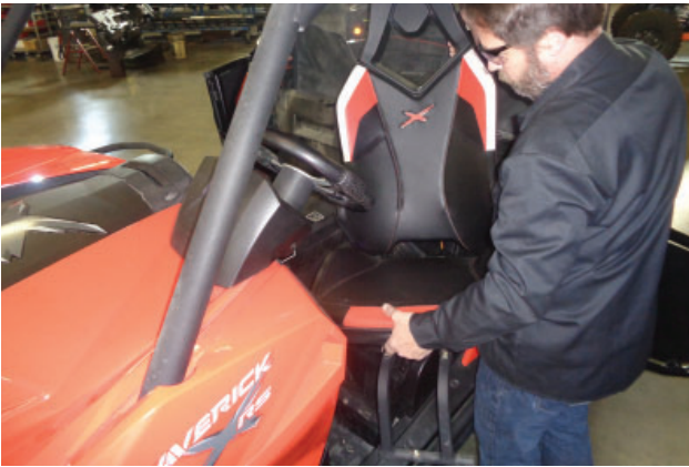
49. Install driver seat back into vehicle.
