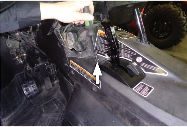
42. Fasten console top driver side using push pins (x3) (removed step 8). Then install front shift gate screw to secure shifter stick assembly.
