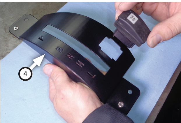
20. Insert override switch assembly into dust cover (4) as shown.
