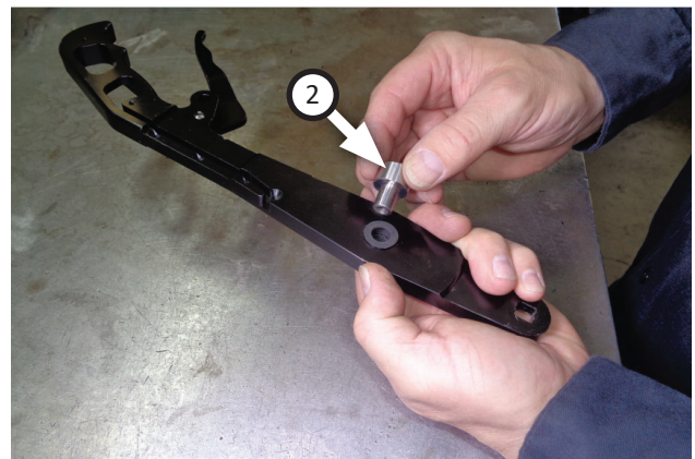
23. Insert pivot sleeve (2) into plastic bushing from passenger side of gated shifter stick.
