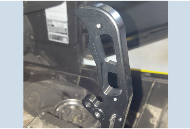
24. Disassemble screws (x4) (12), left (5) and right (6) shifter plates and retain them for later use.
