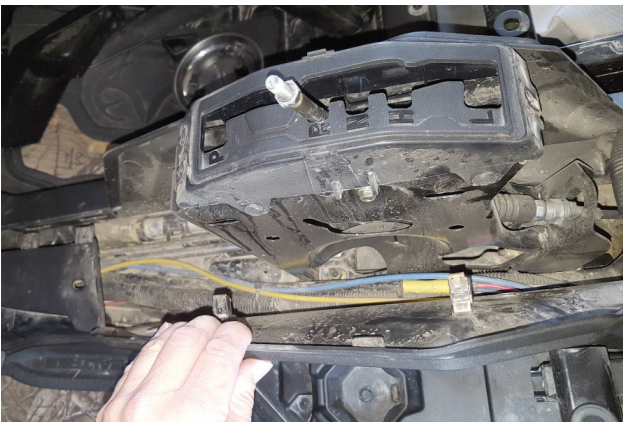
7. Remove driver and passenger console side covers. Retain them for re-install.
