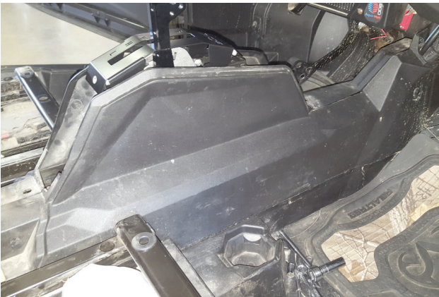
26. Re-install driver and passenger console side covers (removed step 7). Re-install fasteners (x5) (removed step 6).
