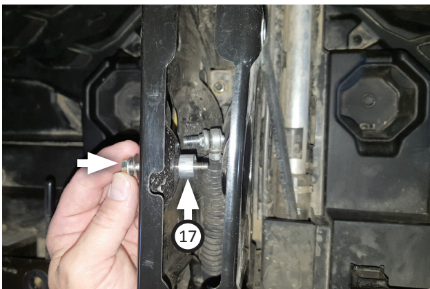
14. Insert shifter bolt and flat washer (removed step 10) in through driver side shifter frame and spacer (17).
