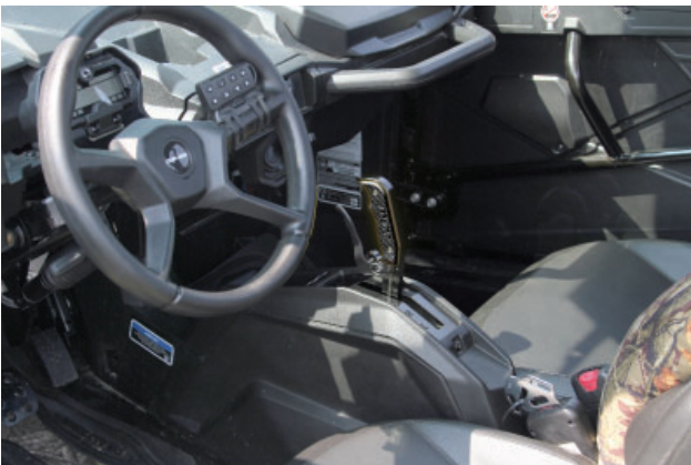
Congratulations, the installation of your XDR Off-Road Magnum Grip Shifter kit is now complete!
