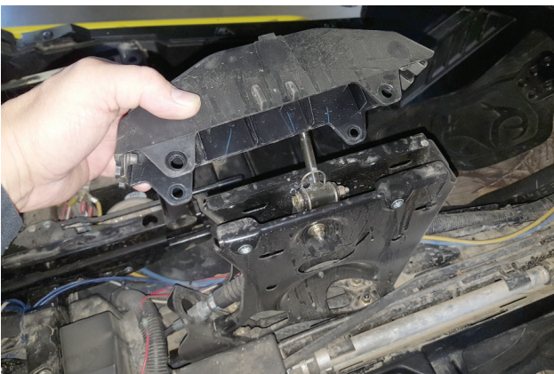
8. Remove screws (x4) and factory shifter dust cover from shifter. Retain screws for later use.
