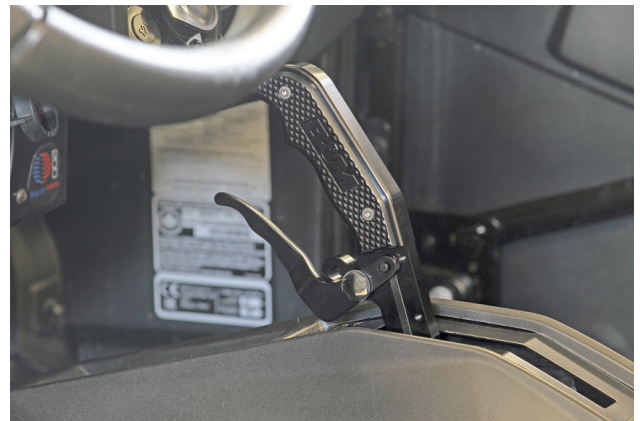
29. Re-install both shifter plates and screws (x4) (removed step 24). Then re-install lever, spring washer and bolt (removed step 23).
