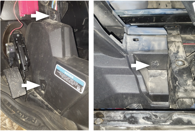
6. Remove fasteners (x5) from driver and passenger console side covers. Retain them for later use.
