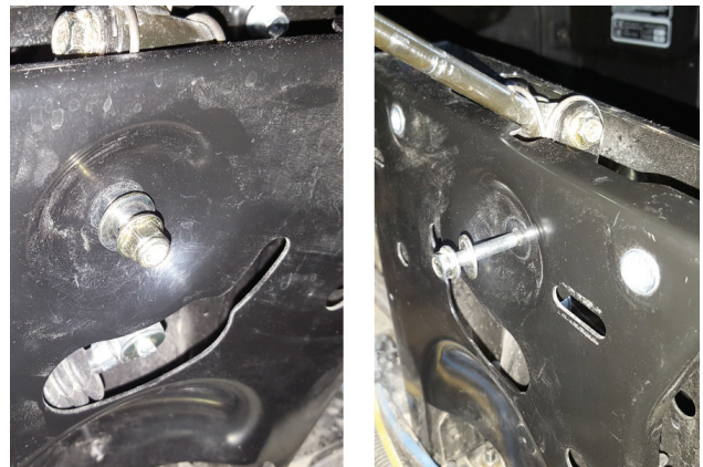
10. Remove shifter bolt, flat washers (x2) and nut. Retain them for later use.
