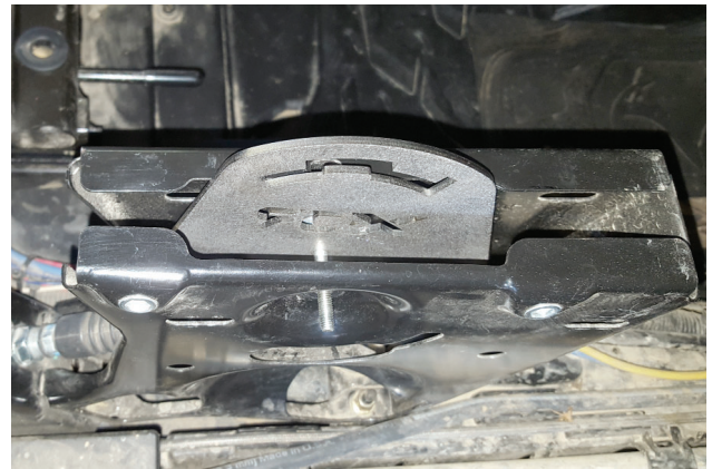
15. Place gate plate (2) into shifter frame and slide shifter bolt through it then out passenger side.
