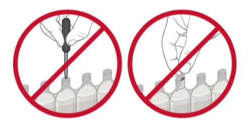
Do not puncture the foil seal or remove it prior to filling a dry AGM battery.
