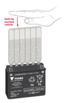
9. Carefully remove the empty electrolyte container from the battery. Fully insert the strip of sealing caps (previously removed from the electrolyte container) into the battery filling ports. Make sure the strip of caps is fully inserted and flush with the top of the battery. Insert the caps by hand, do not use a hammer or excessive force. *Never remove the strip of caps or add water or electrolyte to the battery during its service life*.
